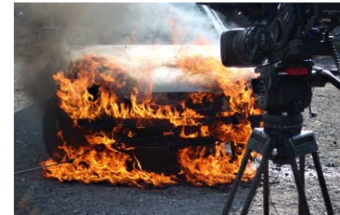
Burning vehicle after leakage of 1234yf in the engine compartment. Photo: wm-punkt/DUH
