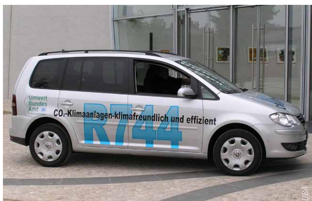
Official car of the Federal Environment Agency with MAC system based on CO 2 .
